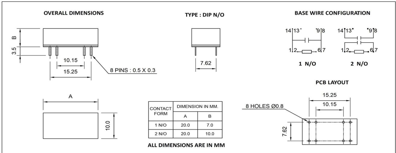
\* Relay Size For 1 N/O 48 VDC will Remain Same as 2 N/O 48 VDC .
